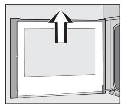
Then pull the inner pane together with the drip channel up out of the plastic runners.
